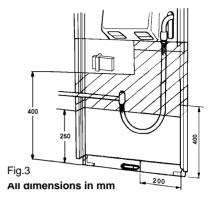
IMPORTANT: FLEXIBLE TUBING USED MUST COMPLY WITH BS. 669 CURRENT EDITION. L.P.G. FLEXIBLE CONNECTIONS MUST BE OF A TYPE SUITABLE FOR L.P.G. AND CAPABLE OF OPERATION UP TO 50MBAR AND TO CARRY A RED STRIPE, BAND OR LABEL.
